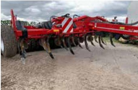
Figure 1: Fully assembled test cultivator
