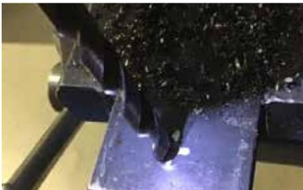
Figure 3: Integrated LED work light. The work area is brightly illuminated.
