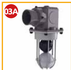
Primary Overflow Valve - Two Balls Code 6100200030-Ø76 Code 6100200025-Ø80 Code 6100200026-Ø100 Iron ring to be welded Weight: 13,9/14,0 kg
