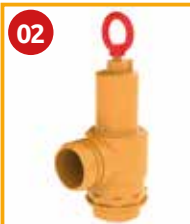
02 Overpressure Safety Valve - 1 1/2 Code 5100200010 Setting range: +0,3 bar / +1,5 bar Working temperature: -20°C / +90°C Thread: G 1 1/2 Weight: 1,02 kg
