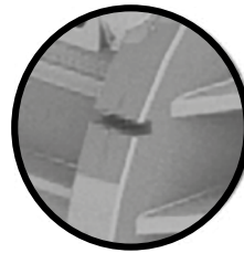
Cut for aligning flange with pump body
