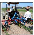
Attachment in the back with hand steering tool gives the possibility of very precise steering.
