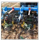
The K.U.L.T. Kress Fingerweeder can be attached to every common cultivator
